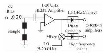
FIG. 2. Schematic of noise measurement apparatus.
