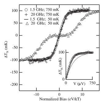
FIG. 4. Variation of differential noise  $\Delta T_N$  with temperature. The differential noise at 1.5 GHz (full line) and 20 GHz (triangles), for a mixing chamber temperature of 50 mK, are plotted vs the dimensionless voltage in units of kT, along with corresponding data for 750 mK (circles and crosses, respectively). Inset shows a comparison of 1.5 GHz data for 750 mK with shot noise theory [full line, Eq. (1)] and electron-heating theory (dotted line).
