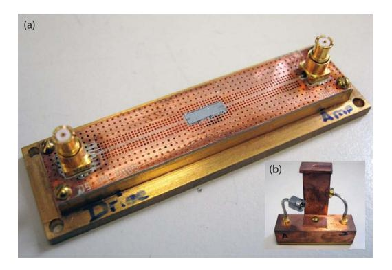
**Figure 5.12: Coffin box holder.** (a) The sample is placed into a 2 mm by 7 mm pocket located in the center of the PCB. The PCB connects to semirigid coasxial cables via SMP surface mout connectors using a bullet. Vias are drilled into the PCB and copper plated to connect the top and bottom ground planes. (b) Inset shows the entire rectangular coffin box with SMA to SMP jumpers.
