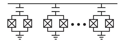
**Figure 3.5: Quantum bus coupling cartoon.** A quantum bus coupling attempts to use a separate quantum degree of freedom. Schematically, it has its analog in a classical instruction bus, with multiple bits locked into the same bus. Here, we can imagine the capacitive coupling of multiple charge qubits to a some feedline which will contain the quantum bus.
