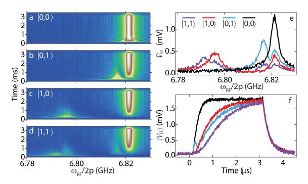
**Figure 8.8: Measurement transients for joint readout.** Transmitted  $V_{\rm H}$  amplitude as a function of time and cavity drive frequency  $\omega_{\rm RF}$ , for computational basis states (a)  $|0, 0\rangle$ , (b)  $|0, 1\rangle$ , (c)  $|1, 0\rangle$ , and (d)  $|1, 1\rangle$ . (e) Time average of the  $V_{\rm H}$  transients in (a–d) over the first 500 ns. (f) Transients of  $V_{\rm H}$  for  $\omega_{\rm RF}$  at the cavity frequency corresponding to  $|0, 0\rangle$ .
