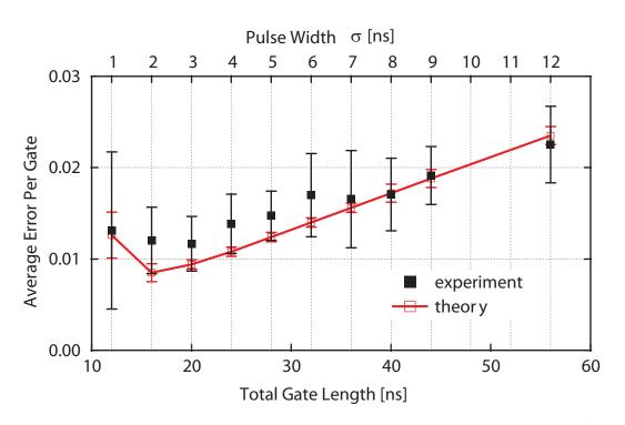
Figure 6.15: Error per gate versus pulse width. Average error per gate (experimental and theoretical) at different pulse widths. The rise for  $\sigma < 2$  ns corresponds to the onset of limitation by the third level of the transmon. The increase in error per gate for  $\sigma > 2$  ns is due to the limitation by relaxation.
