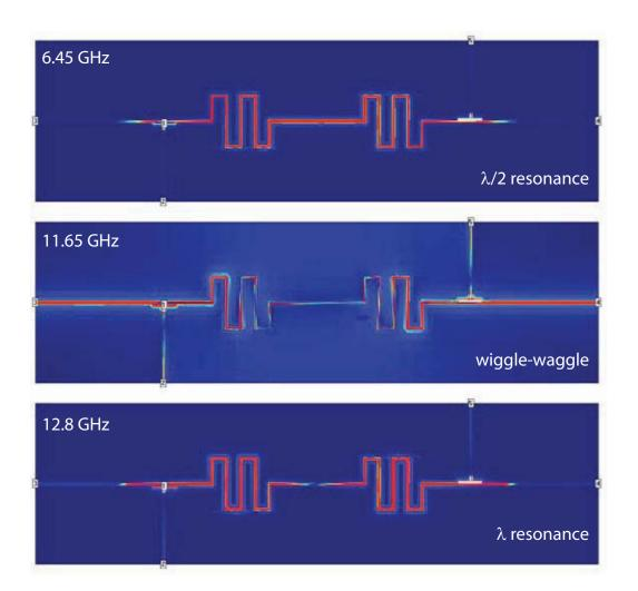
Figure 5.8: Current density simulations of resonators with FBLs. Color scale shows the current density across the chip. Blue represents no current and red represents high current. For the  $\lambda/2$  and  $\lambda$  resonances, we can see the radiation along the center pin and, coupled through only the input and output capacitances on each end. However, for the wiggle-waggle resonance, there are high current paths along the flux-bias lines and all along the center-pin.
