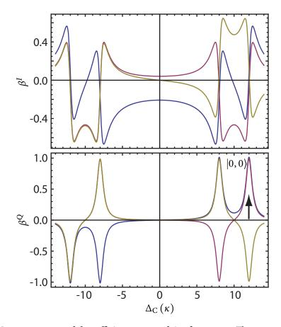
**Figure 4.7: Measurement model coefficients versus drive frequency.** The measurement model coefficients for *ZI* (blue), *IZ* (purple), and *ZZ* (gold) as a function of detuning  $\Delta_{\rm C}$  from the bare cavity frequency. Here the measurement model is broken down into the two cavity quadratures, *I* and *Q*. The cavity is assumed to have a linewidth  $\kappa$ , and the simulation is performed assuming  $\chi^{(1)} = 10\kappa$  and  $\chi^{(2)} = 2\kappa$ .
