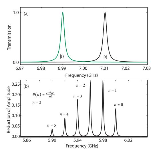
Figure 3.9: Strong dispersive regime of circuit QED. (a) Theoretical state dependent cavity transmission reveals two Lorentzian peaks for the case of  $|0\rangle$  and  $|1\rangle$ , separated by  $2\chi$  (Here assuming  $\chi/\pi = 20$  MHz). (b) Qubit spectroscopy shows multiple peaks corresponding to different cavity-photon number. The weighting of these peaks is given by a simple Poisson distribution as a function of the mean number of photons in the cavity  $\bar{n} = 2$ .
