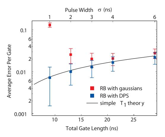
Figure 6.23: Error per gate with derivative pulse shaping. Extracted error per gate versus total gate length with (blue square markers) and without (red square markers) the derivative pulse shaping. We find that with the derivative shaping, an excellent agreement with the simple theory (black solid line). The minimum error per gate of 0.007 ± 0.006 is reached at  $\sigma = 1$  ns.
