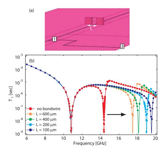
Figure 5.9: Pushing up the wiggle-waggle with bondwires. (a) Schematic for Sonnet simulation incorporating and on-chip air-bridge for connecting the upper and lower ground planes at the center of the CPW. *L* is the length of such a bridge. (b) Simulated  $T_1$  curves for resonator with FBLs and on-chip air-bridge with varying *L* from 600  $\mu$ m to 100  $\mu$ m. With decreasing *L*, the wiggle-waggle resonance is pushed up in frequency.
