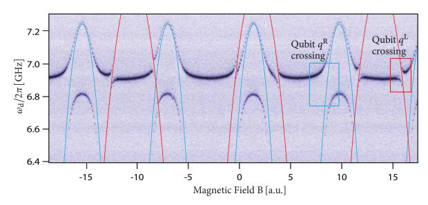
**Figure 6.3:** Transmission versus magnetic field and drive frequency. Although the sample cQED187 is a two transmon device, the strong driving vacuum Rabi experiment is performed on only one of the transmons, specifically investigating the splitting shown in the red box, around magnetic field B = 15.
