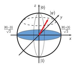
**Figure 2.1:** The Bloch sphere. Geometrical representation of the state space of a single qubit (two-level quantum system). The state of the qubit is represented by the Bloch vector, which is a unit vector within the sphere, describe by two numbers,  $\theta$  and  $\phi$ .
