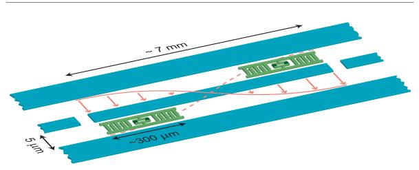
**Figure 3.7: Illustration of circuit QED.** A two-level atom passes through a Fabry-Perot cavity over a transit time *t*, during which the atom undergoes a coherent interaction with photons contained in the cavity with a strength *g*. Photons can leave the cavity at a rate  $\kappa$  and the atom decays via non-cavity modes at a rate  $\gamma$ .
