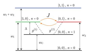
**Figure 4.3: Scheme of the virtual photon swap interaction.** When the qubits are detuned from the cavity  $(|\Delta^{(1),(2)}| \Rightarrow g^{(1),(2)})$  the qubits both dispersively shift the cavity. The excited state in the left qubit  $|1, 0\rangle \otimes |n = 0\rangle$  interacts with the excited state in the right qubit  $|0, 1\rangle \otimes |n = 0\rangle$  via the exchange of a virtual photon  $|0, 0\rangle \otimes |n = 1\rangle$  in the cavity.
