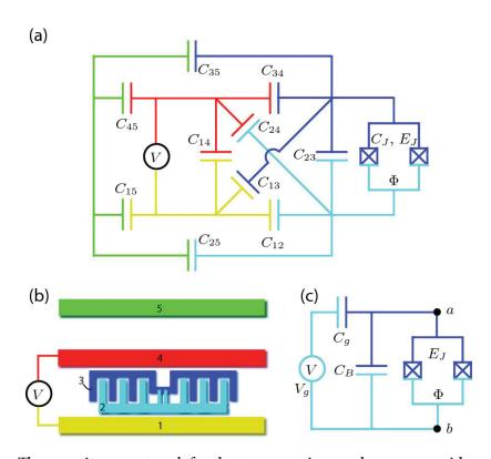
**Figure 5.4:** The capacitance network for the transmon in a coplanar waveguide resonator. a The complete circuit diagram, showing all the capacitances, designed and parasitic, between the 5 metallic areas of the transmon-cavity circuit, shown in **b** (not to scale). **c** The simplified equivalent circuit which can be found by using the electrical engineer's rules for series and parallel capacitors. (Figure used with permission from [61]. See Copyright Permissions.)
