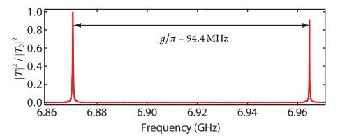
**Figure 6.1: Vacuum Rabi splitting.** When the qubit is in strong coupling with the cavity, the cavity transmission undergoes a splitting into two peaks, separated in frequency by  $g/\pi$ . Shown here is the normalized transmitted homodyne amplitude as a function of applied frequency, with the vacuum Rabi peaks split by 94.4 MHz. This splitting is associated with one of the qubits in sample cQED187.
