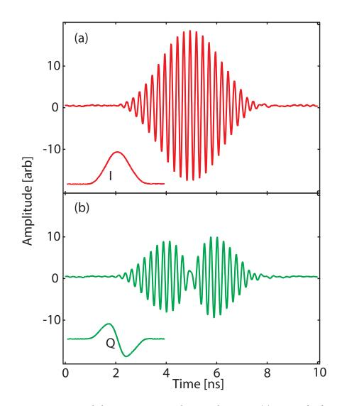
**Figure 6.19:** Gaussian and derivative on I and Q quadratures. (a) A standard truncated Gaussian is applied on one quadrature. (b) Frequency modulated truncated derivative of Gaussian is applied on the other quadrature. The pulse shape is shown in the lower left corner.
