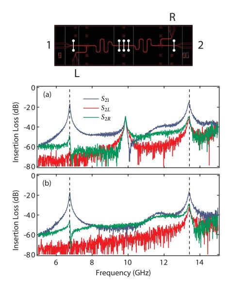
Figure 5.14: Resonator with FBL in octobox. With additional wirebonds, the transmission spectrum is further improved to (a). However, there is still a strong resonance in all 3 measurements at  $\sim$  10 GHz, corresponding to a 3 dimensional cavity mode. This is suppressed with the use of the flip-chip and filled octobox design, with which we measure the transmission spectra shown in (b).
