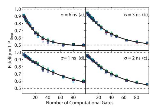
Figure 6.21: Randomized benchmarking for various pulse widths using derivative pulse shaping. Total average fidelity and averaging just over the Pauli randomizations for  $\sigma = 6, 3, 2, 1$  ns having implemented derivative pulse shaping. The error per gate decreases monotonically with decreasing  $\sigma$ .
