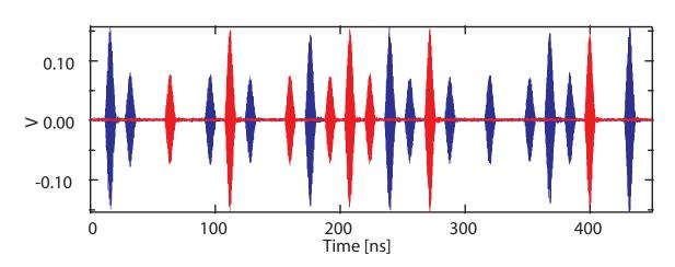
**Figure 6.7: Sample sequence of concatenated pulses.** Example of a sequence of concatenated pulses for randomized benchmarking section 6.3.6. Blue (red) pulses are x(y) gates of either  $\pi$  or  $\pi/2$  rotations. The longest applied sequences consist of ~ 200 gates.
