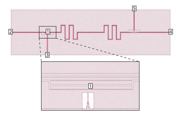
**Figure 5.6:** FBL schematic for Sonnet simulations. For performing the Sonnet simulations, a simplified chip and transmon design is used. We label 5 ports, and find the total admittance referenced to port 1, where the transmon qubit is located.
