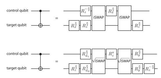
Figure 2.5: Circuit form for constructing a *c*NOT from an *i*SWAP or  $\sqrt{i$ SWAP gate. When the accessible two-qubit interaction is *XY* and not *ZZ*, the natural two-qubit entangling gates are either the *i*SWAP or  $\sqrt{i}$ SWAP. Creating a *c*NOT gate then requires the concatenation of at least two of each of the gates, combined with multiple single-qubit rotations around various directions.
