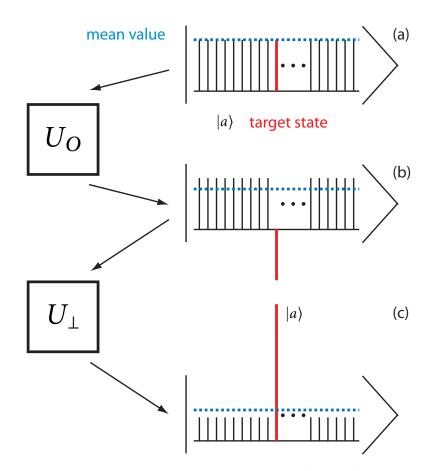
Figure 2.9: Cartoon state illustration of Grover iteration. The search space starts off in an equal superposition of all states in the qubit register Hilbert space as in (a). The appropriate oracle  $U_0$  for finding target state  $|a\rangle$  is applied, inverting the phase of only  $|a\rangle$ .
