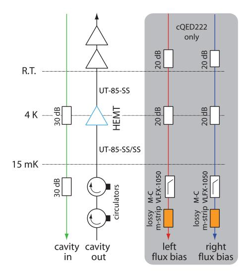
**Figure 5.15: Schematic of cryogenic circuitry.** There are a total of four cryogenic lines: input, output, left flux-bias and right flux-bias. The experiments for cQED157 and cQED187 do not employ the FBLs.
