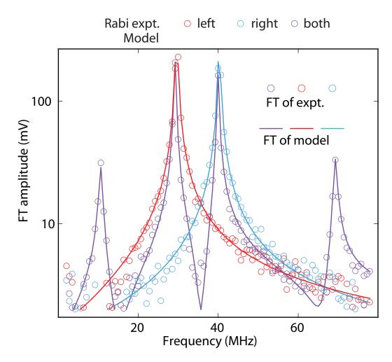
**Figure 8.10:** Fourier transforms of Rabi oscillations. Fourier transform (FT) of the three Rabi experiments (circles) and of best fits (lines). While the red (blue) traces show one main peak at the Rabi frequency  $\Omega^{L(R)}$ , the purple traces reveal peaks at  $\Omega^L$ ,  $\Omega^R$ ,  $\Omega^L + \Omega^R$ , and  $\Omega^L - \Omega^R$ , demonstrating the mixing property that makes the joint measurement sensitive to qubit-qubit correlations.
