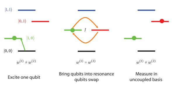
Figure 7.9: Coherent swap protocol. Three step process for performing coherent swaps.
