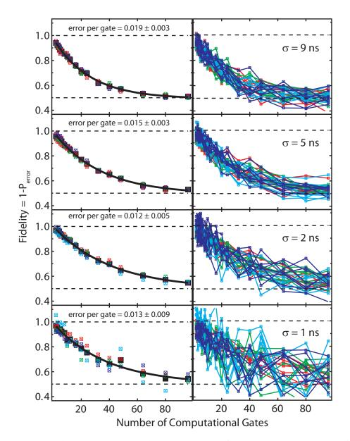
**Figure 6.14:** Trace by trace randomized benchmarking. The average error per gate is shown in the left panels for  $\sigma = 9$ , 521 ns. The 32 unique trace-by-trace realizations are shown for the same  $\sigma$  in the right panels. We can see the increase in the spread of all the traces at the shortest pulse lengths, reflected in the increase in the error bars of the extracted error per gate.
