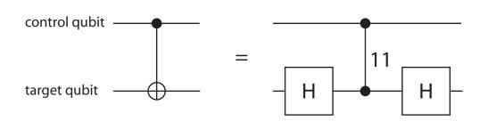
Figure 2.4: Circuit form for constructing a *c*NOT from a *c*-Phase gate. A *c*NOT gate can easily be constructed from the *c*-Phase gate  $cU_{11}$  by performing single-qubit Hadamard gates on the target qubit before and after.
