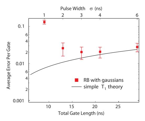
**Figure 6.17:** Error per gate with normal pulse shaping. Extracted error per gate versus total gate length using Gaussian pulse shapes. There is a sharp rise in the error per gate at  $\sigma = 3$  ns. The solid line is a simple two-level system model taking into account the relaxation of the qubit.
