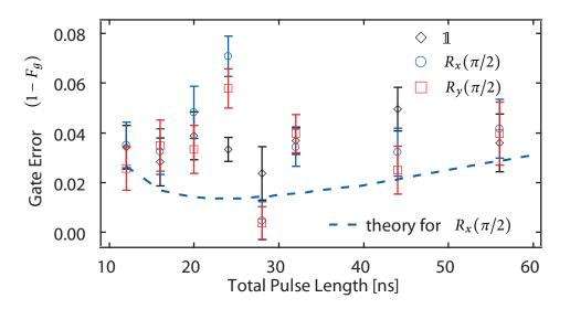
**Figure 6.11: Gate errors from QPT.** Gate error vs. total pulse length obtained from quantum process tomography plotted for the three processes  $1, R_x(\pi/2), R_y(\pi/2)$
