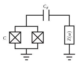
**Figure 3.10:** Environmental coupling of transmon. The voltage relaxation rate of the transmon qubit can be found from a simple *RC* decay time. The transmon capacitance *C* is coupled to an environmental impedance of  $Z(\omega)$  through a coupling capacitor  $C_q$ .
