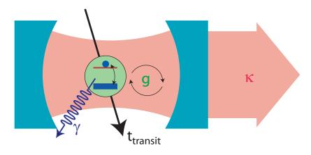
**Figure 3.6: Illustration of cavity QED.** A two-level atom passes through a Fabry-Perot cavity over a transit time *t*, during which the atom undergoes a coherent interaction with photons contained in the cavity with a strength *g*. Photons can leave the cavity at a rate  $\kappa$  and the atom decays via non-cavity modes at a rate  $\gamma$ .
