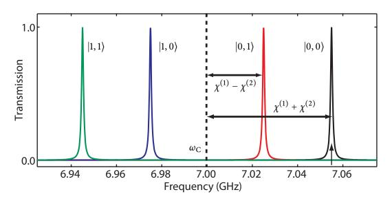
Figure 4.6: Transmission in strong dispersive regime for two qubits. The four dispersive shifted cavity transmission peaks for a two-qubit and cavity system with a bare transmission frequency of 7 GHz, and qubits with dispersive shifts  $\chi^{(1)}/2\pi = 40$  MHz and  $\chi^{(2)}/2\pi = 15$  MHz.
