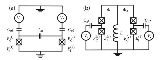
Figure 3.3: Superconducting charge qubit coupling schemes. (a) Fixed capacitive coupling. A mutual capacitance  $C_m$  connects two CPB circuits, resulting in an always-on interaction. (b) Tunable inductive coupling. Two split-CPB circuits are joined by a mutual inductance L, which allows independently tunable loops via external magnetic fluxes  $\Phi_1$  and  $\Phi_2$ .
