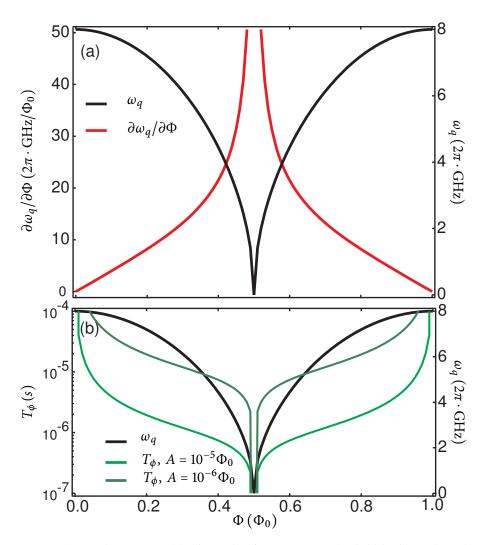
**Figure 3.11:**  $T_{\phi}$  **due to flux noise.** (a) The qubit frequency  $\omega_q$  (solid black) and its derivative with respect to flux  $\partial \omega_q / \partial \Phi$  (solid red) are shown versus flux  $\Phi$ . (b) Assuming a flux noise spectrum amplitude  $A = 10^{-6} \Phi_0$ , the inferred flux-dependent  $T_{\phi}$  (solid green) is plotted versus  $\Phi$ .
