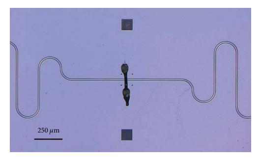
**Figure 5.10: Optical image of an on-chip wirebond.** Wirebonds across the center pin are generally  $200 - 300 \,\mu$ m long. In standard practice, we place 3 wirebonds in parallel.
