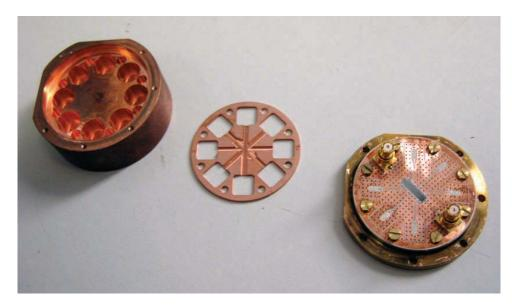
**Figure 5.13: Octobox holder.** The far left is the copper octobox which permits 8 connections to a sample. This particular copper octobox is designed to fill up the entire space in between the box and the sample lid. The piece in the middle is the "flip-chip" which is similar in size to a PCB, but made out of copper with traces milled out to avoid shorting to transmission lines on the PCB. The piece on the right is the lid with 8-port PCB but only a two-port sample attached.
