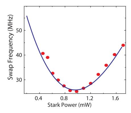
**Figure 7.11:** Stark swap frequency. By repeating the Stark swap protocol for various powers  $P_{AC}$ , we are able to extract the frequency of the oscillations (red points) and map out the same avoided crossing with splitting 2*J* as in figure 7.8, which is shown in the solid blue curve.
