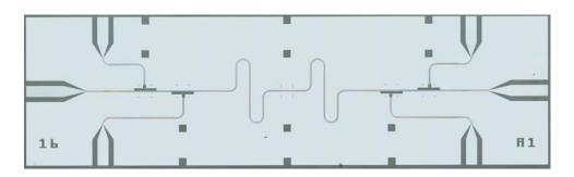
**Figure 10.1:** Four qubit circuit QED sample. New four qubit circuit QED samples places two qubits on each end of the resonator. The device is now a 6 port device, as there are now 4 flux-bias lines for each of the qubits, in addition to the input and output ports of the resonator.
