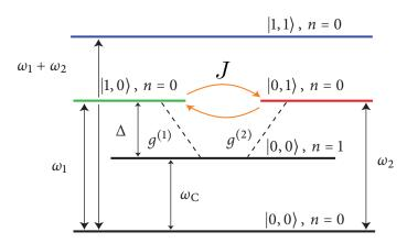
**Figure 7.4: Scheme of the virtual photon swap interaction.** When the qubits are detuned from the cavity  $(|\Delta^{(1),(2)}| \Rightarrow g^{(1),(2)})$  the qubits both dispersively shift the cavity. The excited state in the left qubit  $|10\rangle \otimes |n = 0\rangle$  interacts with the excited state in the right qubit  $|01\rangle \otimes |n = 0\rangle$  via the exchange of a virtual photon  $|00\rangle \otimes |n = 1\rangle$  in the cavity.
