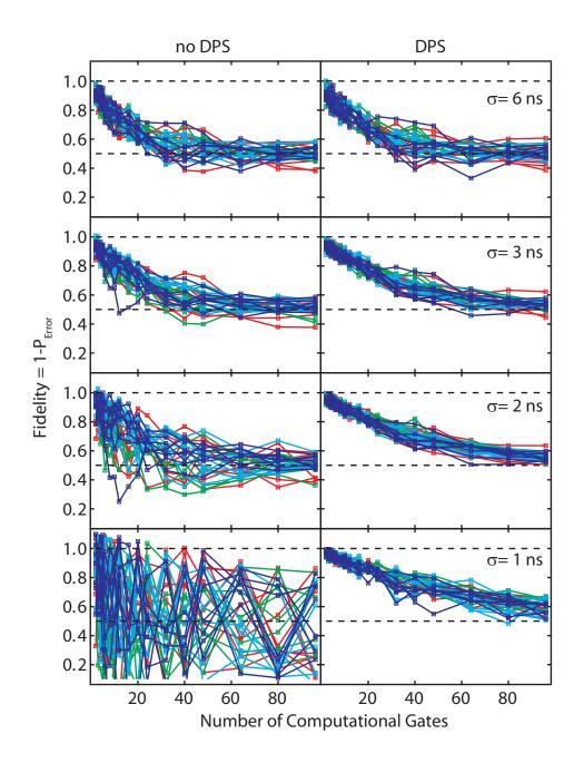
**Figure 6.22:** Trace by trace with and without derivative pulse shaping. All unique 32 randomized traces with and without the derivative pulse shaping for  $\sigma = 6$ , 3, 2, 1 ns. The spread in the traces can be seen to get visibly worse without the shaping, and visibly better with the shaping.
