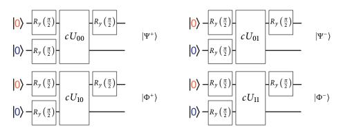
Figure 8.7: Experimental protocols for generating Bell states. Gate sequence generating twoqubit entanglement. Starting from  $|0, 0\rangle$ , simultaneous  $\pi/2$  rotations on both qubits create an equal superposition of the four computational states. A c-Phase  $cU_{ij}$  then phase shifts  $|i, j\rangle$  in the superposition and produces entanglement. A final  $\pi/2$  rotation on  $Q_L$  evolves the entangled state into one of the four Bell states depending on the  $cU_{ij}$  applied.
