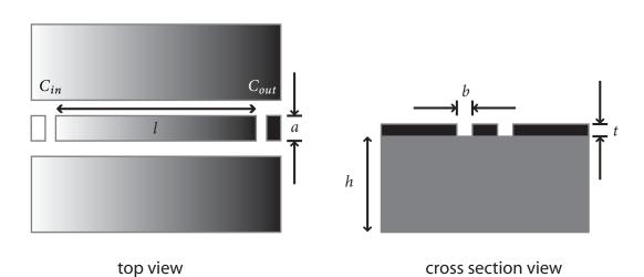
**Figure 5.1: Coplanar waveguide geometry.** The frequency of the CPW resonator is defined by the length of the center pin between the gap capacitors at each end. The center pin width is given by *a* and the gap between the center pin and ground planes is *b*. The ground planes are designed to be much wider than *b* in order to be effectively infinite.
