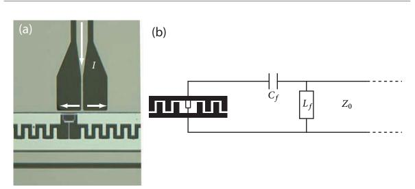
**Figure 5.5:** The flux-bias line. (a) Optical image of the flux-bias line short-circuited termination near the SQUID loop of the transmon qubit. (b) Modeling the flux-bias line as a circuit-decomposition, with a capacitance in series  $C_f$  with the transmon, and a shunt inductance  $L_f$ . The inductance is accounted for by the 2  $\mu$ m by 20  $\mu$ m short-circuited termination to ground.
