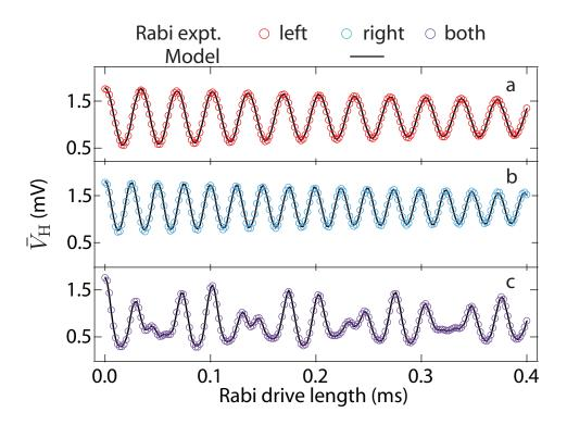
**Figure 8.9: Rabi experiments for readout characterization.** Rabi oscillations on the (a) left qubit, (b) right qubit, and (c) simultaneously on both. Solid lines are fits to the model in (8.5).
