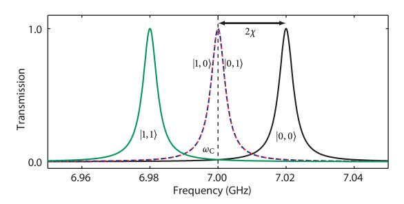
Figure 4.8: Dispersive peaks for generating Bell states by measurement. When the two qubits have equal dispersive shifts  $\chi$ , the cavity transmission peaks corresponding to  $|01\rangle$  and  $|10\rangle$  overlap. Then a measurement tone on this cavity peak would project onto a Bell state.
