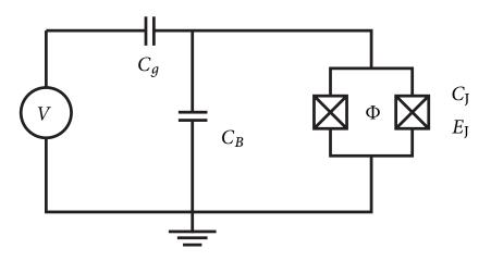
**Figure 3.8: Reduced transmon coupling to CPW schematic.** The transmon is coupled to the CPW transmon line via a gate capacitance  $C_g$ . A split pair of junctions with  $E_J$  and  $E_C$  are in parallel with a shunt capacitance  $C_B$ .
