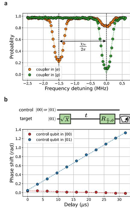
FIG. 6. **Measuring interaction strength for the CZ gate.** **a.** Spectroscopy on the target qubit cavity with the coupler either in the ground (green) or excited state (orange). **b.** Circuit diagram for the Ramsey sequence on the target dual-rail and the associated phase shift as a function of delay time with the control qubit cavity either empty (red) or occupied with a photon (blue).
