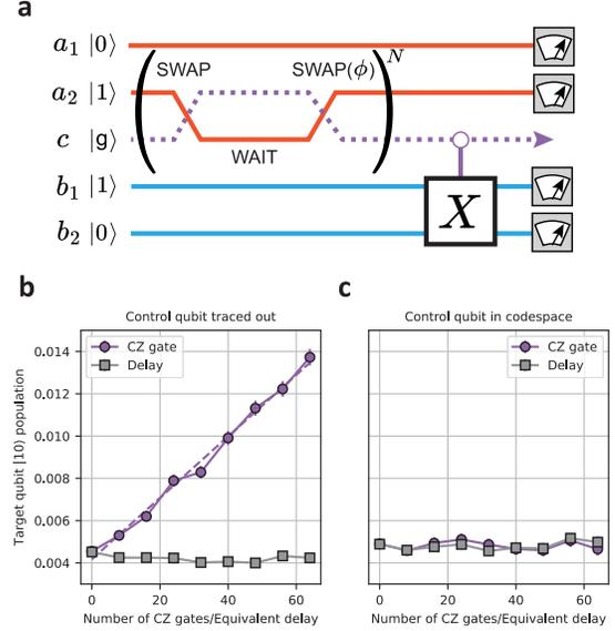
FIG. 8. **Residual coupler excitation** **a.** Pulse level protocol used to map the residual coupler population into target qubit. **b.** Target qubit  $|01\rangle$  population as a function of number of CZ gates in the sequence or delay when the control qubit measurement outcome are traced out **c.** Same as **b** but when control qubit measurement outcomes are postselected to be in the codespace.
