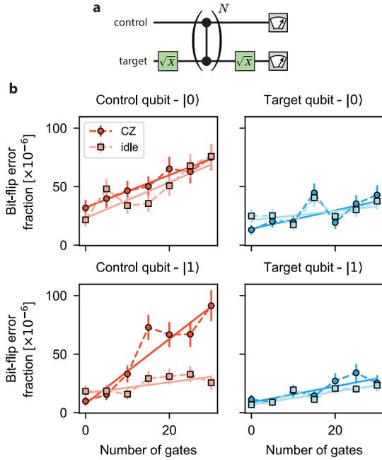
FIG. 9. **Measuring bit-flip errors during CZ gate a.** Circuit used to measure bit-flip errors **b.** Results of bit-flip measurements for the various combinations of initial logical states of the target and control dual-rails, compared to the idling states when no CZ gates are performed. The extracted linear trends (solid lines) are used to produce the quantities presented in Fig. 3f.
