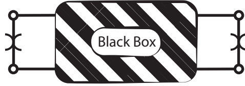
Figure 3.6: Black-box quantization with multiple qubits. We assume the black-box to be described by an n -by- n matrix Z(\omega) , where the spider element for each of the n junctions sees a different port.
