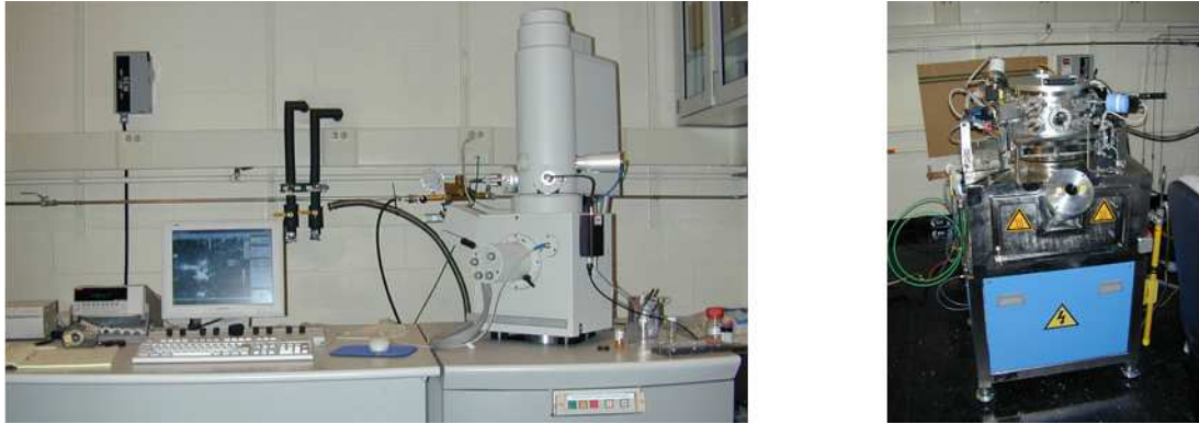
Figure 5.11: a) An FEI XL30 Sirion scanning electron microscope. It is capable of 4 nm viewing resolution, and has been modified with the Nanometer Pattern Generation System NPGS to allow it to act as electron beam lithography tool. It has successfully been used to write features as small as 40 nm, well beyond the requirements of this project. b) A custom made (by Plassys ) electron beam evaporator. It is capable of depositing aluminum, gold, copper, titanium, chrome, and alumina. It features a stage which can be rotated about two axes to allow multi-angle depositions. This feature is used to create the overlap junctions and to control the edge profile of aluminum resonators. It is a load locked system which can pump down to \sim 1 \times 10^{-7} .
