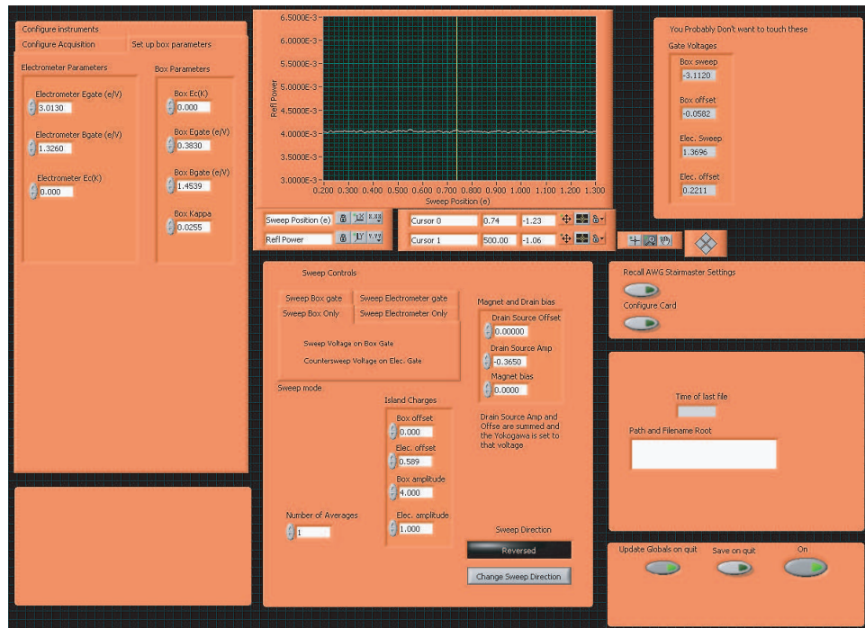
Figure 5.15: Screenshot of the “stairmaster”, which allowed real time variation of sweeps that could be isolated to only the box or the SET islands.
