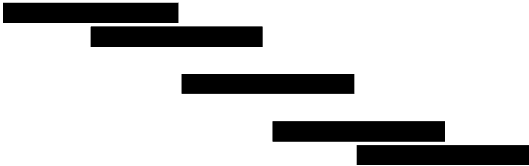
Figure 6.7: The schematic layout of an edge coupled microstrip bandpass filter.
