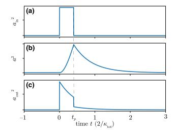
FIG. 6. Dynamics of a resonant ring-down measurement: (a) the incoming field  $a_{\rm in}$ , (b) the cavity-mode amplitude a, and (c) the outgoing field  $a_{\rm out}$  as a function of time. Not to scale.
