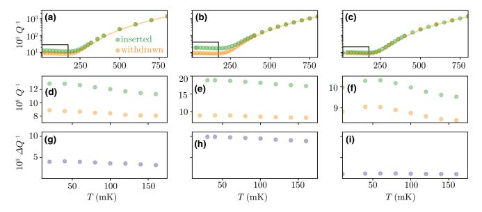
FIG. 9. Temperature sweeps. The measured internal loss  $Q^{-1}$  with the sample withdrawn (orange) and inserted (green) as a function of the mixing-chamber plate temperature, for (a) 100- $\mu$ m-thick EFG sapphire, (b) 460- $\mu$ m-thick EFG sapphire, and (c) 440- $\mu$ m-thick HEMEX sapphire. The orange lines are fits to Mattis-Bardeen theory [50], as described in the supplement of Ref. [36].
