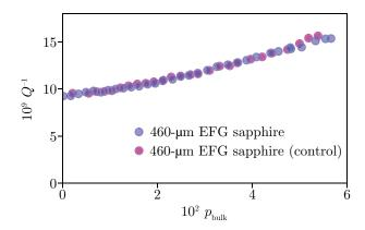
FIG. 10. Position sweeps on nominally identical samples. The position sweep in Fig. 4 is repeated with a second piece of 460-μm-thick EFG sapphire denoted as a control. The control is prepared in nominally the same way but is cut from a different wafer of the same material.
