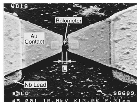
FIG. 1. SEM photo of the diffusion-cooled bolometer.
