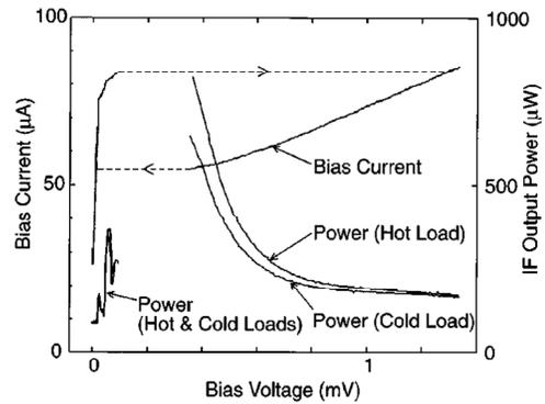
FIG. 2. The current–voltage ( $I$ - $V$ ) curve for the bolometer with local oscillator power applied. The dashed lines show the regions in which switching occurs. The device resistance is negative below about 0.4 mV. The normal resistance  $R_N$  is  $20 \Omega$ . The if output power is shown for both a hot (295 K) and a cold (77 K) load in the receiver signal path.
