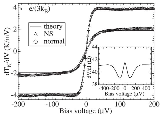
FIG. 2. Differential shot noise  $dT_N/dV$  vs bias voltage for an N-S device at  $T = 70$  mK and for the same device driven normal ( $T = 100$  mK) and the theoretical predictions with no adjustable parameters. The inset shows the differential resistance of the device vs bias voltage at  $T = 70$  mK.
